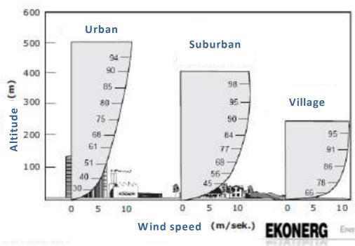
The picture shows an increase in wind speed with height for three basic types of terrain: a city with tall buildings, suburban area with low houses and the lowland village.
